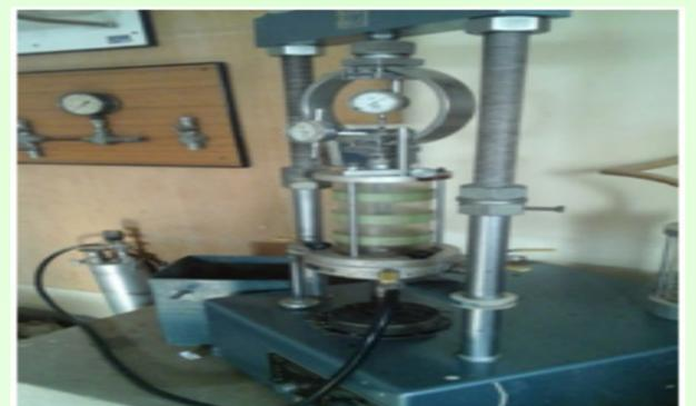
California Bearing Ratio (CBR) Test Equipment
