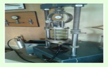
California Bearing Ratio (CBR) Test
