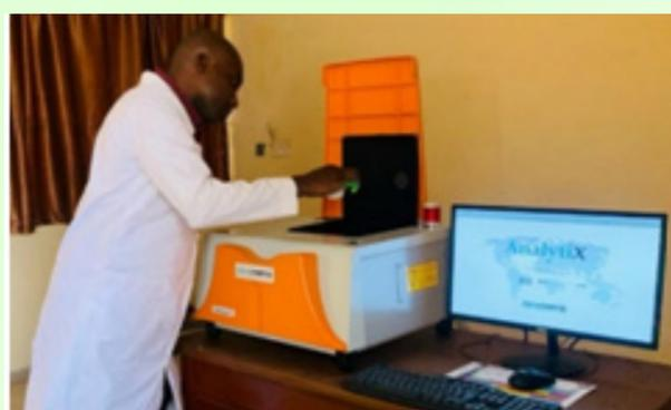
Genius IF Xenometrix XRF Equipment
